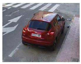
**Solution:** It seems that LP is well lit and readble by eye. However, if we'll measure full frame in photoshop, we will see that LPR width is under 100px which is not enough. License plate width in the frame should be increased and be at least 130 pixels.
