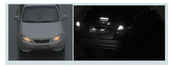
**Solution:** Not sufficient light degrades recognition performance. The camera must be configured to night mode. Should be used an infrared light.
