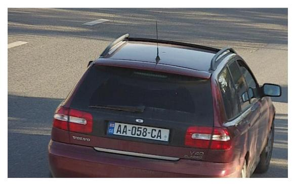
**Solution:** Notice the license plate tilt angle. License plate tilt angle must be within +/-5 degrees.
